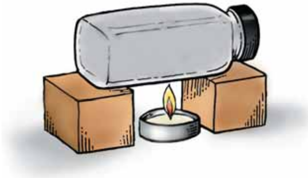
Figure 16.1 The setup for the rheoscopic fluid
